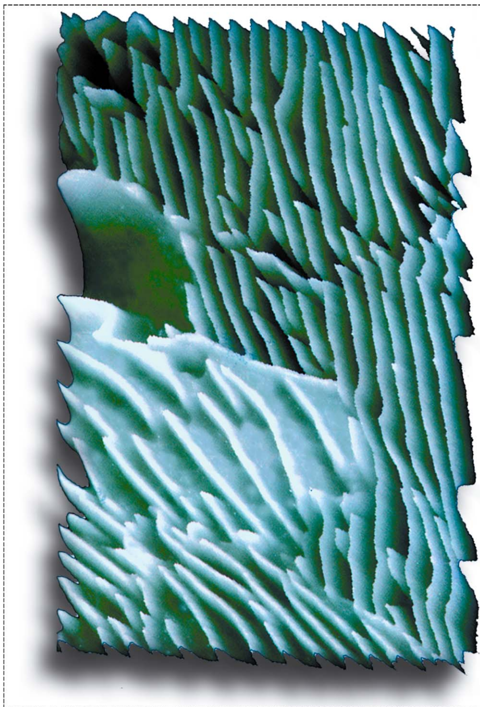
Figure 2 AFM picture of the pearlitic microstructure of a eutectoid steel, patented and cold-drawn. The sample was etched; valleys were filled with ferrite, and the ridges are of cementite, in some places plastically deformed. The height of the ridges is about 200 nm (courtesy of B. Monteiro).
